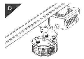
D. Once assembly is complete, turn on track power and turn the intensity knob on the light fixture to confirm it is operational.
